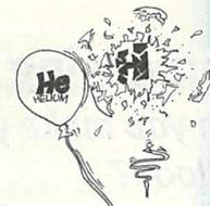
*Non stretch balloons filled with lifting gas.* As they rise in the air the gas in the balloon expands and is released from a special one way valve. These balloons are effected by the sun which warms the gas inside causing it to expand and be released. At sunset these balloons will fall because the lifting gas cools and exerts less pressure.
